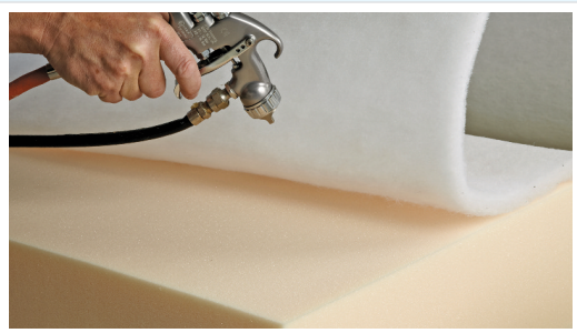
Polyester fibre being fitted to the top and bottom surface of a foam seat cushion.
