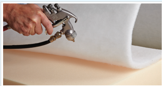
Polyester fibre being fitted to the top and bottom surface of a foam seat cushion.
