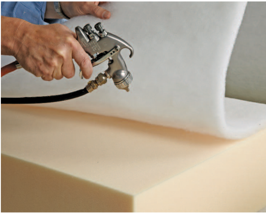
Polyester fibre being fitted to the top and bottom surface of a foam cushion.
