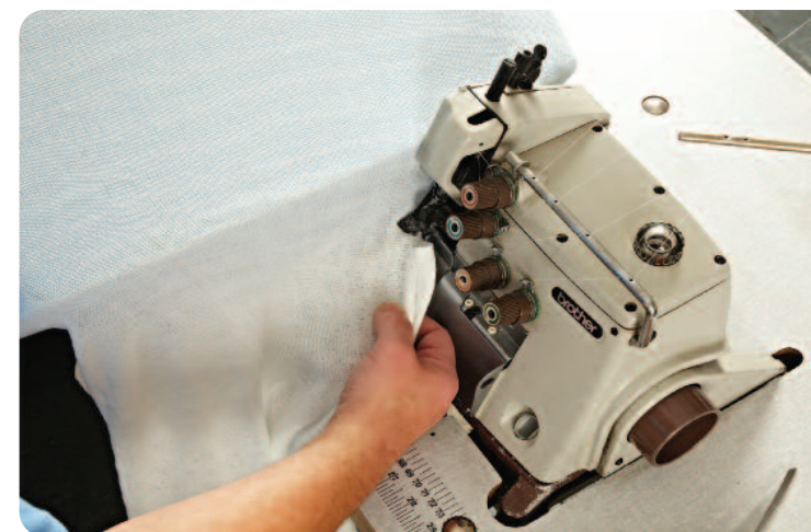
Machine Closing a Stockinette under cover.
