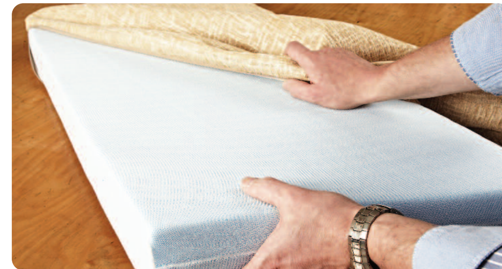
Fitting a stockinette covered interior.
