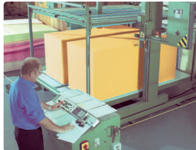
Cutting a Superior Foam block.
