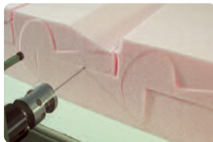
Profiling Superior Foam shapes.
