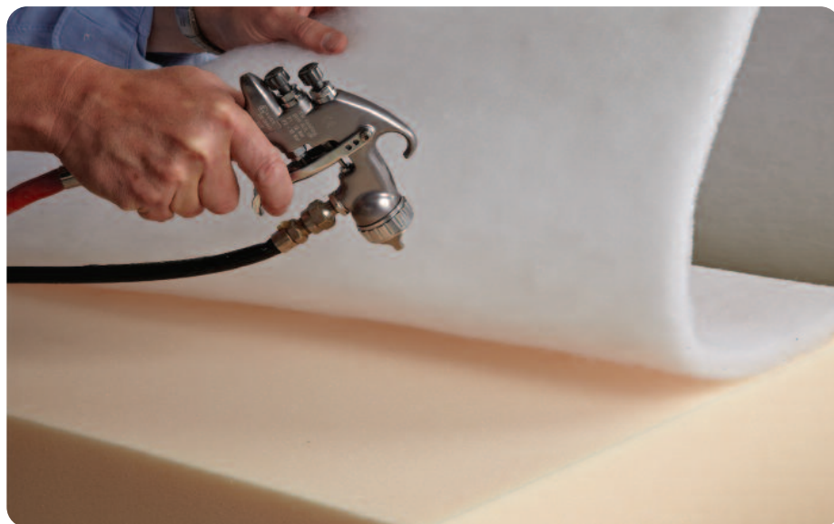
Polyester fibre being fitted to the top & bottom surface of a foam cushion.
