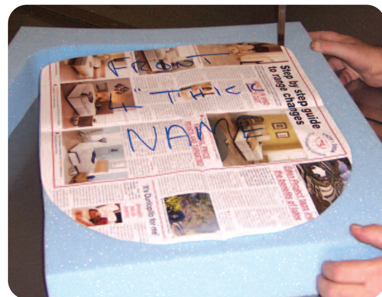
Cutting Classic Foam to a customers own template.
